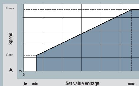
Speed setting for speed control via set value voltage interface 0 to 10 V DC.
