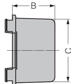
The protective cap cannot be mounted with motor VDC-3-43.10! When using the protective cap, power is reduced due to the thermal conditions.
