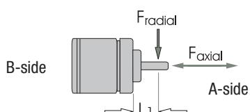
The point of application of the axial load is defined as the centre point of the shaft (A-side, both directions) and for the radial load, it is the distance from the A-sided flange to the point of entry, defined as  $L_1$ .
