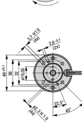
Blind holes for self threading screws according to DIN 7500
