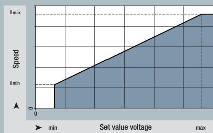
Speed setting for speed control via set value voltage (interface 0 to 10 V DC).
