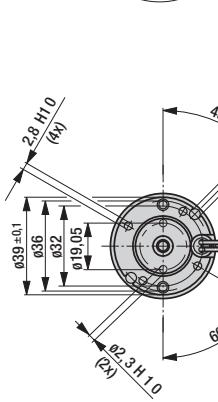
Blind holes for self threading screws according to DIN 7500
