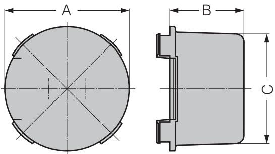
The protective cap cannot be mounted with motor FDC-3-43.10! When using the protective cap, power is reduced due to the thermal conditions.
