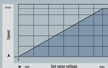
Speed setting for closed loop speed control using set point voltage (0 to 10 V DC interface)
