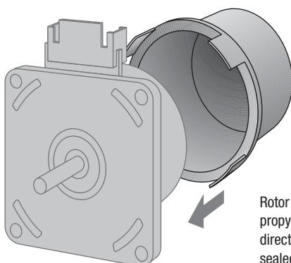
Rotor protective cap of black polypropylene (PP). The cap is fitted directly onto the motor flange and sealed with a rubber seal.
