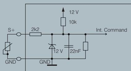
Typical wiring of the reference input with the voltage controlled version. Special features are contained in the relevant data sheets.
